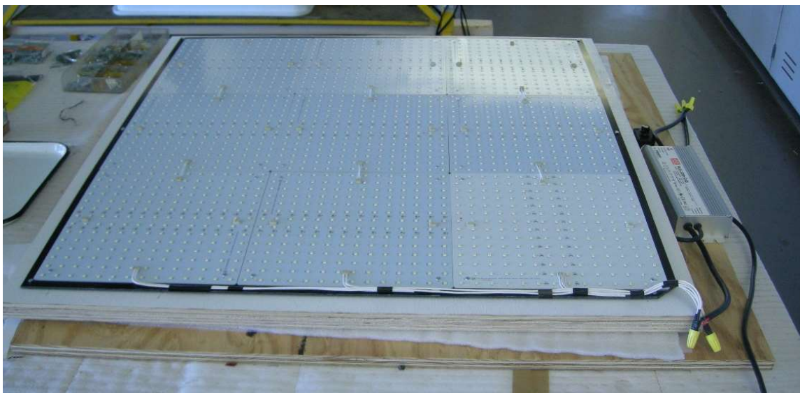
LED light panel built into the new framed wood enclosure
